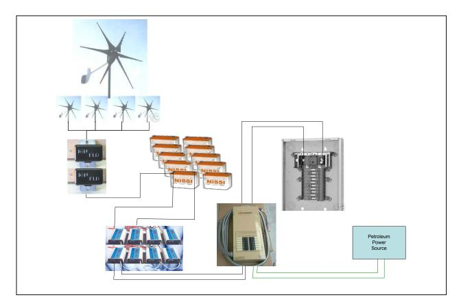
Beginning with the wind generators, 4 Hornet Power Systems SC120 turbines are utilized to
