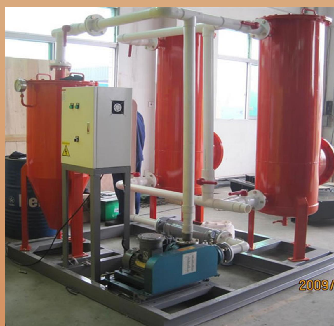
Low cost high production scrubber systems, clean Bio-Gas to pipeline grade methane for sale to commercial distribution companies.
